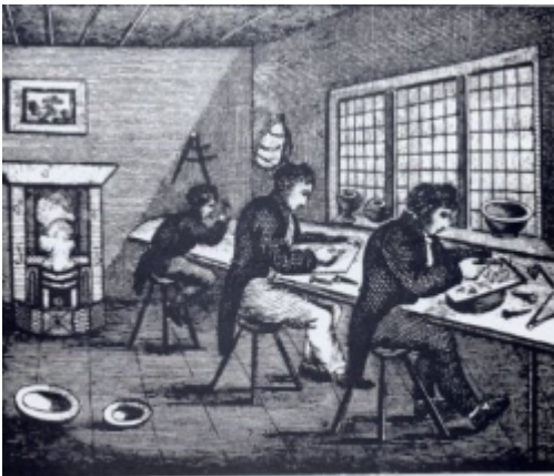
Engraving designs on Copper Plates, for producing the much admired 'blue printed pots': &c.
